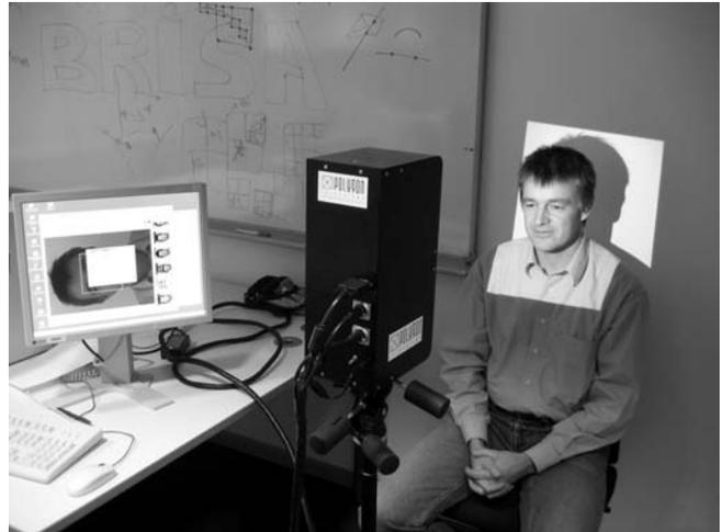
**Fig. 1.** Active acquisition device for three-dimensional face scanning
