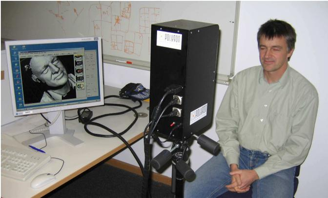
Fig. 1. Capture device (left) and three-dimensional face scanning (right)
